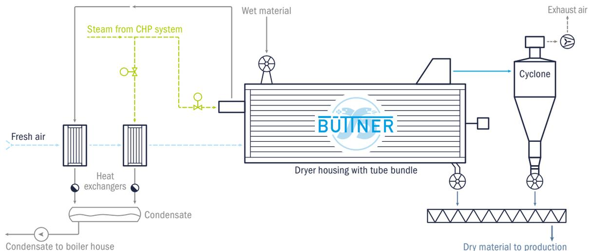
The product to be dried enters a stationary casing with a rotating tube bundle through an air-tight rotary valve. Depending on capacity, the dryer can be used as either a single or double rotary bundle dryer.
